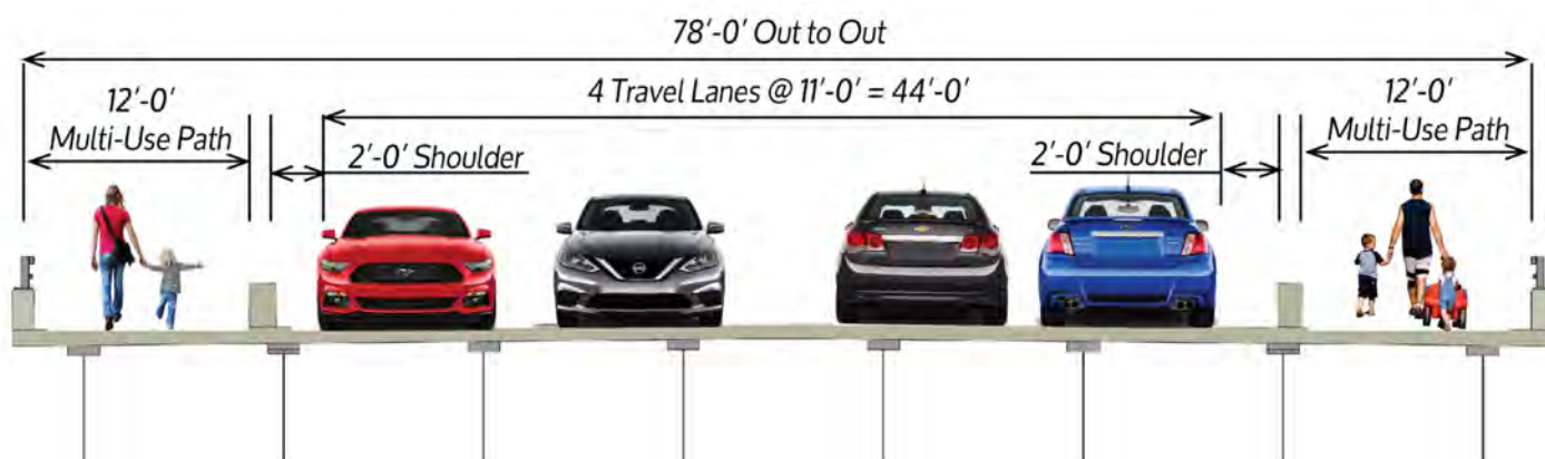
Fig. 8 - Proposed Bridge Typical Section
